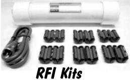
To make solving RFI problems easier, we have assembled kits of parts that you will need. Each kit contains a Line Isolator<sup>tm</sup>, a 3foot deluxe jumper cable and six RFI cores. Caution: In mobile installations, it is not safe to use your radio equipment when your vehicle is in motion. RFI can effect the vehicle's onboard computer.
