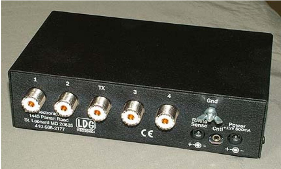
The 2.5 x 5.5 mm jack coaxial DC power connector is on the right. The ground connection is via the wingnut. The radio sense input is a second 2.5 x 5.5 mm coaxial jack, and the control cable is a 1/8" stereo jack; the control cable is included with the DTS-4R remote.
